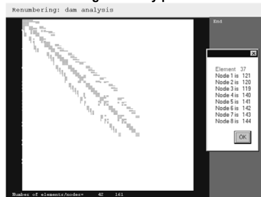
Figure 3 Display of global stiffness matrix structure during assembly process
